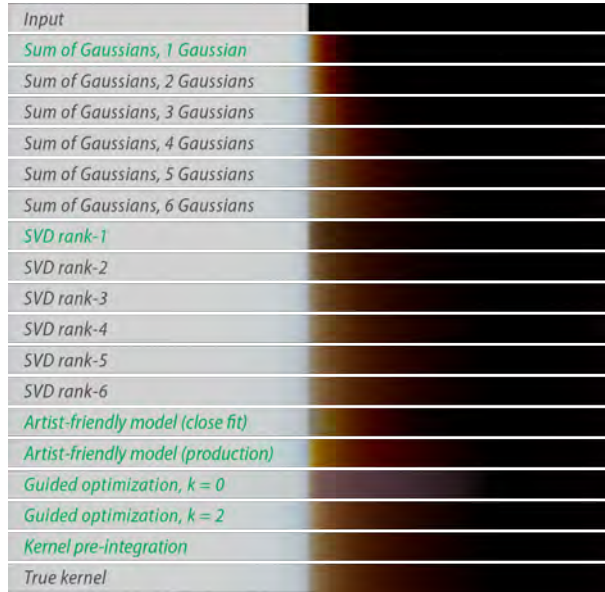
Figure S.3: Our results reveal that SVD-based low-rank approximations scale better with the number of convolutions than the state of the art [dLE07], however, they still yield only a coarse approximation of the true kernel in the separable case (rank-1). Note that all separable rank-1 kernels are highlighted in green. The pre-integrated kernel is exact for axis-aligned functions, such as this example. The guided optimization with k = 2 provides a comparably good fit, while the k = 0 case captures the fine details near the boundary at the expense of the far-range scattering quality. A manual approximation using our artist-friendly model is illustrated by two approximations, where for the first (close fit), perceptual similarity to the ground truth was the modeling objective, while the second (production) was tweaked by an artist for production purposes. Additional 2D visualizations of the different kernels are provided in the second supplementary document, where we also demonstrate that the radial asymmetry of the SVD-based kernels vanishes rapidly with increasing rank.
