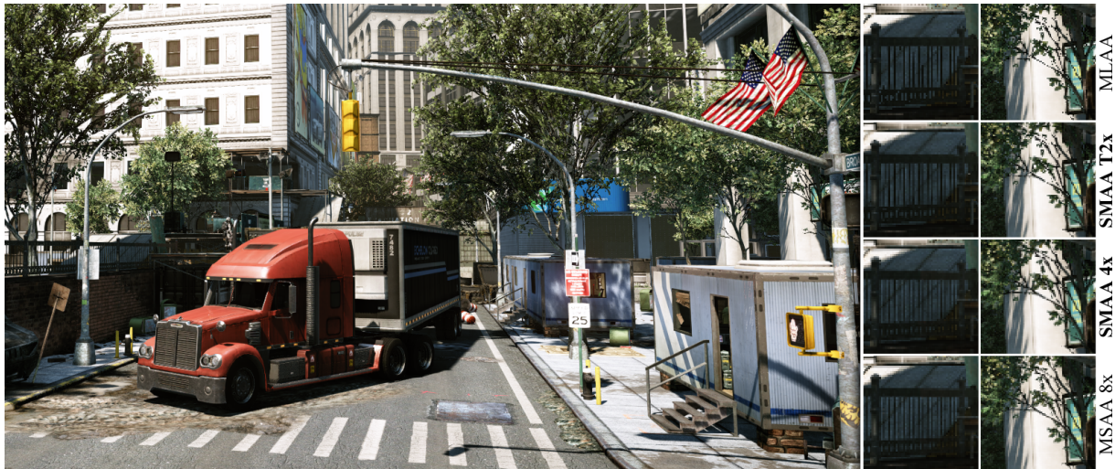
Figure 1: Example of SMAA 4x integrated in the Crysis 2 game. The insets show the differences between MLAA [JME* 11], our novel SMAA T2x and 4x algorithms and MSAA 8x as reference. For 1080p frames, the average cost of SMAA T2x is 1.3 ms and 2.6 ms for SMAA 4x, measured on a NVIDIA GeForce GTX 470.
